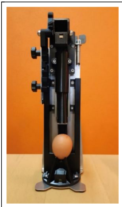
Figure 3. Test stand by Agri Advanced Technologies GmbH with a special fixing system
