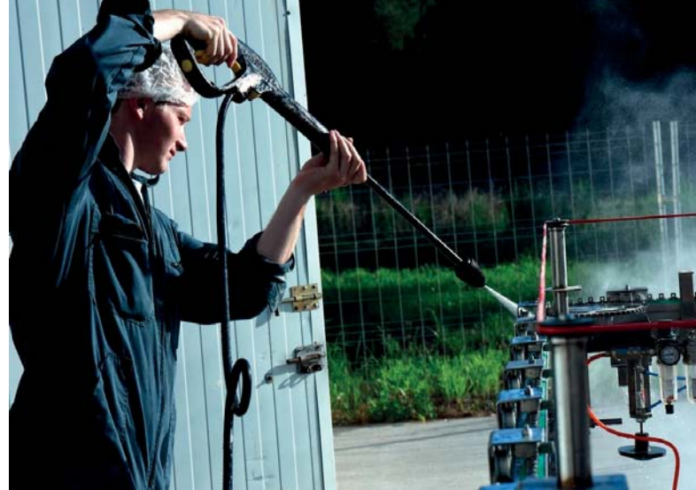
Image 4 - High pressure cleaning of the AAT device
