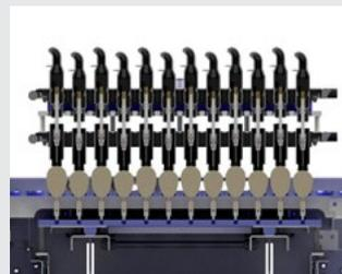
First, the bottom stunning pins penetrate the eggshell and connect with the egg fluid.
