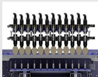
The stunning pin injectors will be positioned and locked. The position depends on the egg size.
